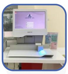
By using LIS (LED Information Service) this unit gives detailed status information to the user about the status of the working process. The workpad distinguishes 3 color modes:
